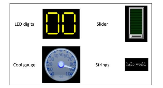
The purpose of this application note is to introduce the use of the basic ViSi-Genie-Raspberry-Pi library functions. The application consists of a 4D Picaso display module displaying four objects – a LED digits, a slider, a cool gauge, and a text string. These objects interact with the Raspberry Pi in a manner illustrated below.
