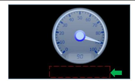
The area inside the red box will be the space occupied by the text string to be displayed. The object can be dragged to any desired location and resized to the desired dimensions. The **Object Inspector** on the right part of the screen displays all properties of the newly created strings object named **Strings0**.
