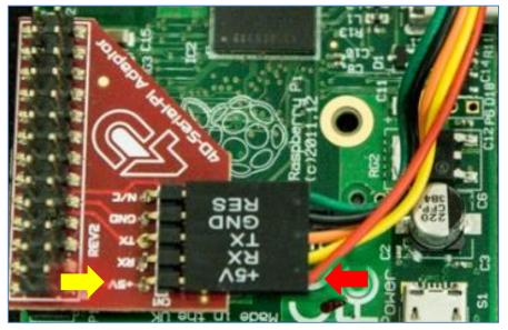
Check the orientation of the 5-way-cable-to-display-module connection.
