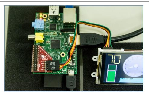
Check the orientation of the 5-way-cable-to-adaptor connection.
