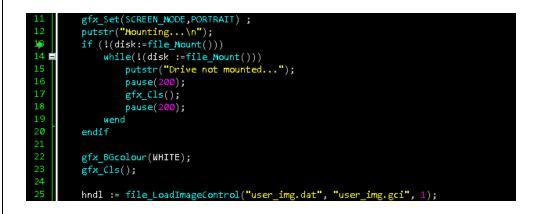
When starting a new project in the ViSi environment these set of statements are already included in the coding area. The last part of these set of statements uses a function file\_LoadImageControl() to call on the object data/information files on the uSD drive. This initializes the data to be called in using the variable 'hndl'. In addition, the filenames for the dat and gci files are automatically changed to the project filename as soon as the project is saved.
