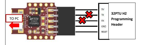
If using COM1 to talk to the uCAM-II, connect the uUSB-PA5 to the programming header H2 of the display in the normal way. In this setup, the display can be programmed while it is connected to the uCAM-II module.
