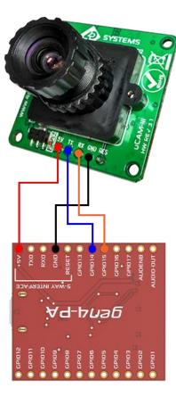
For gen4 display modules, a break out board (gen4-PA/4D UPA) is needed to communicate with the uCAM module.
