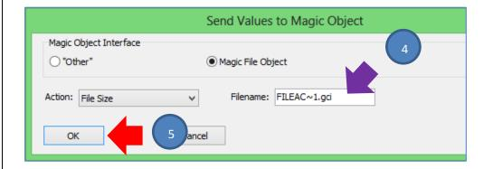
**Note: "FILEAC~1.gci"** is the filename of the generated graphics file for the Workshop example project **"FileAccess.4DGenie"**. When you build this project, Workshop generates the supporting files and their 8.3 format-filenames and copies them to the uSD card. FILEAC~1.gci is one of these files. If the name of the project is different or was changed, replace "FILEAC~1.gci" with the correct or another filename. Make sure that the file exists on the uSD card.
