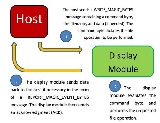
The WRITE\_MAGIC\_BYTES and REPORT\_MAGIC\_EVENT\_BYTES messages or commands are two complementary messages that are used in ViSi-Genie Magic. The host sends a WRITE\_MAGIC\_BYTES message, and the display
