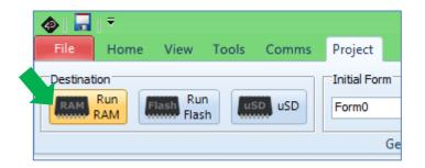
The run-from-RAM or Run RAM option causes the program to be copied (from the flash memory where it resides) to the RAM section and executed from there. The program will run faster in this case, but less RAM space is available to the application since the application code itself occupies a part of the RAM space.
