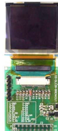
Breakout board with the OLED display, unfolded
