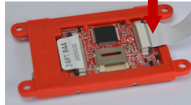
FFC Cable Connected to the gen4-display (Silver Side up)
