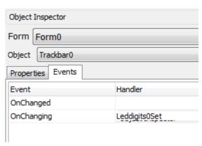
Each time the cursor on the track-bar is moved, the LED digits display is updated accordingly.
