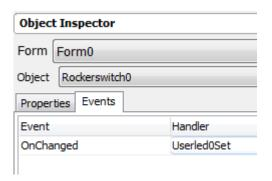
Each time the switch is turned on and off, the LED is updated accordingly.
