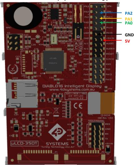
Connect the circuit to the display module accordingly.
