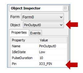
This is because at the start of the program, pin IO3\_PIN is already set to low (**IdleState**). This will disable the display and the uSD card. The user has no way of driving the pin high again since the display is turned off. Due to this, it is therefore strongly recommended for users to know the functions of the GPIO pins of a display module first before using them. Again, a display module's datasheet can be downloaded from its product page at www.4dsystems.com.au.
