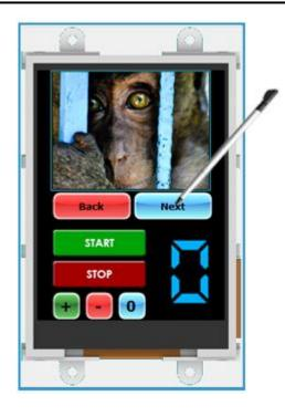
Upon releasing Winbutton1, the second frame of Userimages0 is displayed. Also, a message is sent from the display module to the PC. The message is displayed on the white area on the right part of the GTX Tool window.
