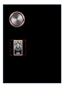
When the program runs, 4dbutton1 will toggle the logic state of pin IO2. To illustrate:
