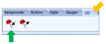
Click on the WYISWYG screen to place the object. The object inspector lists all the default properties of the newly-added pin input object named PinInput0. A pin input object (like a pin output object) will always reside in Form0.
