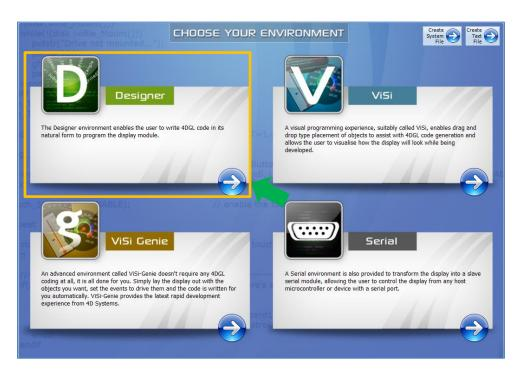
A new project is created. The user can now update the firmware on the display module and can start designing an application as well. Workshop 4 displays a simple 4DGL code which the user can improve.
