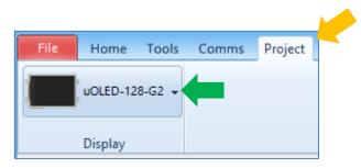
If using a different display module, change the target display module by clicking on the display button.
