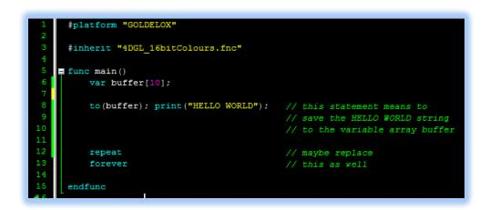
In the above program a variable buffer with an array size of 10 is being declared. The size declaration of the variable array means that there are 10 indexes. In turn each of the index contains a pair of bytes. It may simply be stated that, for this example, each of the array index shall contain 2 characters. Therefore, the total bytes that can be held in an array of this size would be 20.
