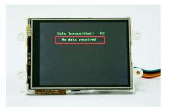
This means that the PIC18F is not connected and that the serial connections are left hanging or disconnected. On the other hand, if we connect the PIC18F to the display module, we will have a result in the display similar to the one below.
