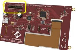
The serial communication port can be assigned to a pin according to the specifications of the DIABLO16 Datasheet. Referring to the image below, we can see that a particular serial transmit or receive pin can only be assigned to a particular pin number. This pin may be common to all the other three serial com ports or exclusive to itself.
