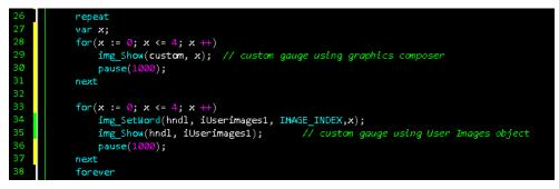
The statements contained inside the repeat-forever loop simply runs both the custom made gauges into a cyclic pattern of changing the IMAGE\_INDEX number from the 0 to 4. Building and downloading the project will result to a screen image
