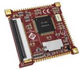
Driving the display and peripherals is the DIABLO16 embedded graphics processor, a very capable and powerful chip which enables stand-alone functionality, programmed using the 4D Systems Workshop 4 IDE Software. The Workshop IDE enables graphic solutions to be constructed rapidly and with ease due to its design being solely for 4D's graphics processors.
