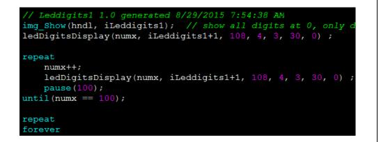
Note that we simply copied the generated ledDigitsDisplay(...) line for Leddigits1 and pasted it inside a repeat-until loop. Recompile the code and download it again to the display module's processor. Leddigits1 should render its frames 0 to 99, which correspond to the values 00.00 to 00.99, respectively.
