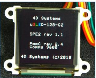
The default baud rate is 9600 and the latest firmware is loaded on to the display. To learn how to modify the default settings, refer to **Section 2.2** (**Additional Configuration Parameters for Serial Communication**) of the Goldelox Serial Command Set Reference Manual.
