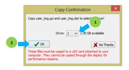
Workshop now copies the graphics file to the  $\mu SD$  card. Properly unmount the uSD card from your PC then mount it to the display module. Note that the filename of the graphics file is derived from that of the project filename. Check the contents of the uSD card for the exact filename of the generated files. There are two files actually – the GCI file and the DAT file. The GCI file contains the actual graphics. The DAT file contains a list of the images inside the GCI file.
