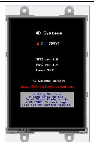
The default baud rate is 9600 and the latest firmware is loaded on to the display. To learn how to modify the default settings, refer to **Section 2.2** (**Additional Configuration Parameters for Serial Communication**) of the Diablo16 Serial Command Set Reference Manual.
