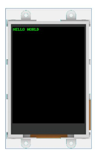
The message area displays the messages sent to and received from the display module.
