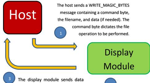
The display module sends data back to the host if necessary in the form of a REPORT\_MAGIC\_EVENT\_BYTES message. The display module then sends an acknowledgment (ACK).
