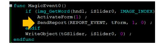
This will cause the program to send a REPORT\_EVENT message to the serial port just after Form1 is activated. For more information about this function, see **section 5.1 Genie Magic callable Functions** of the <u>ViSi-Genie Reference</u> <u>Manual</u>.
