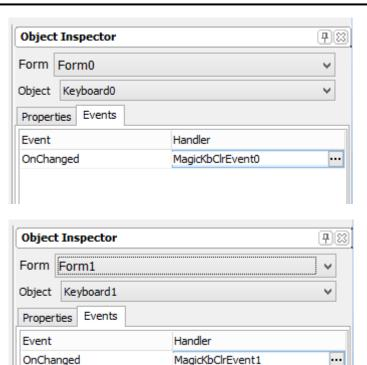
The OnChanged Event of Keyboard0 and Keyboard1 are set to MagicKbClrEvent0 and MagicKbClrEvent1 respectively. This is for MagicKbClrEvent Object to receive key pressed on the keyboard and can be processed later on.
